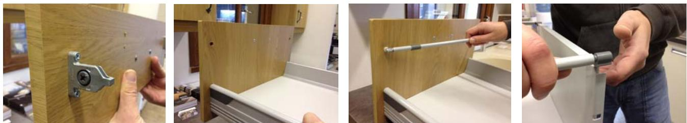
Pan drawers will need a further hole drilling to take the support rods. Using a 10mm drill bit, drill another hole a maximum of 13mm deep.
