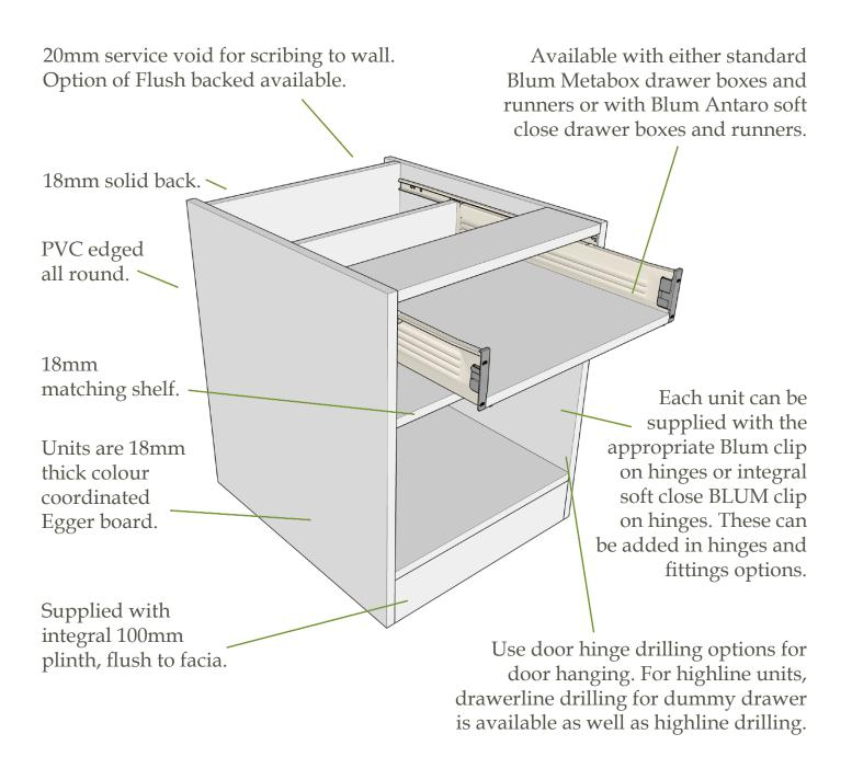
Units are supplied pre-built for durability and easy installation.
