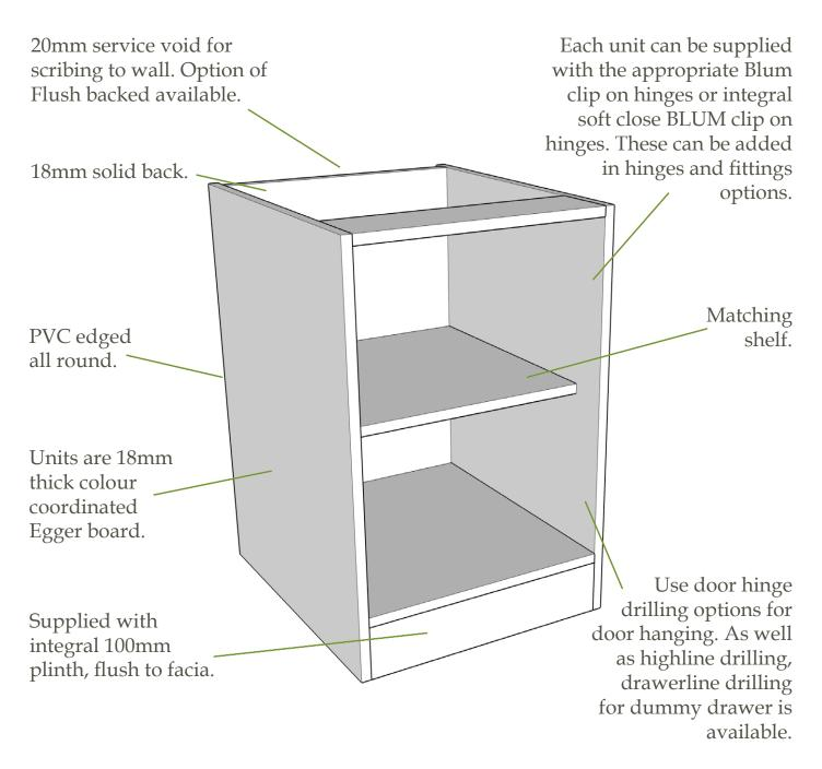
Units are supplied pre-built for durability and easy installation.
