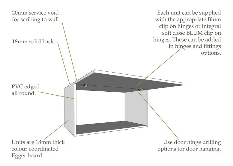
Units are supplied pre-built for durability and easy installation.
