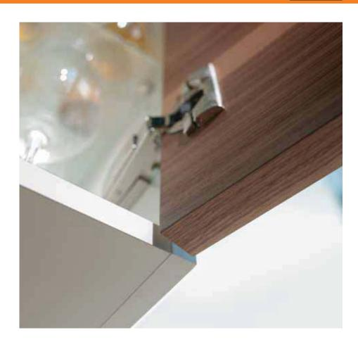
Silent and effortless, that's how cabinet doors close with CLIP top BLUMOTION hinges — regardless of the weight or closing speed. The BLUMOTION soft close mechanism is integrated in the hinge cup, and continues to provide the quality of motion you have come to expect from Blum hardware.
